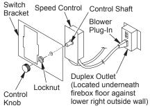
Figure 27 - Attaching Speed Control to Firebox
